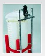
Mixer Mount Assembly A unique mixer mount design can be adjusted to change mixer height for a variety of applications.
